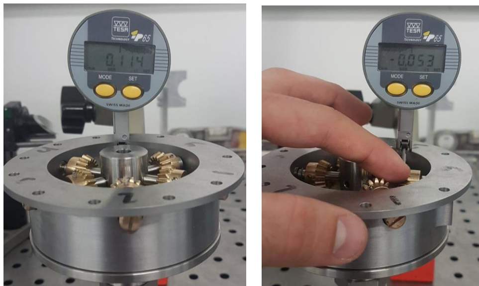
Figure 32: Results obtained for circumferential backlash using a system: without springs (left) and with springs (right)
